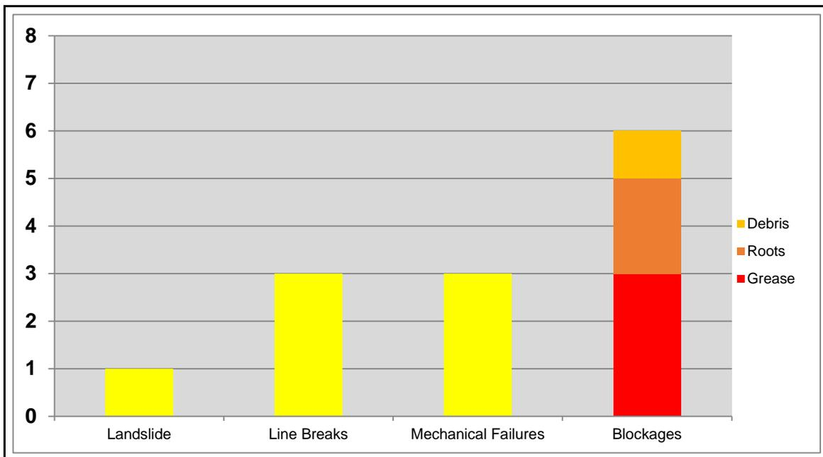
**Figure 2.2 Gallons of SSO due to Operational Issues, per Cause**
